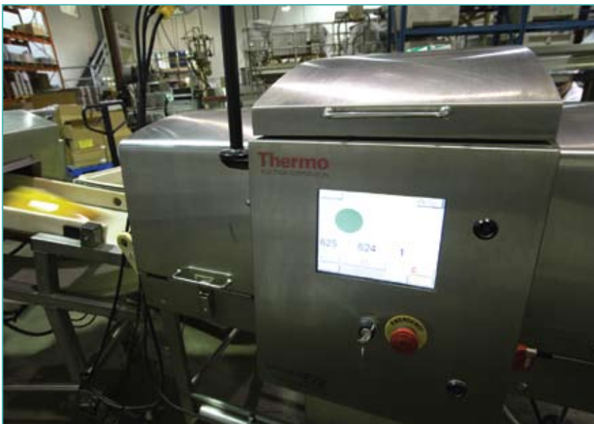
End-of-line X-ray inspection, supported by metal detectors upstream, are becoming more common in food plants. Source: Thermo Fisher Scientific.
