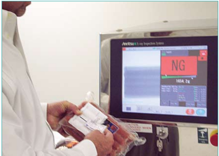
An Anritsu technician holds a 2-lb. package of dinner franks and a 0.7mm fragment of stainless steel that was detected by an X-ray machine, which generated a “no go” message on the display screen. High-speed image processing and increased focus on food safety are winning an expanding role for X-ray inspection.
