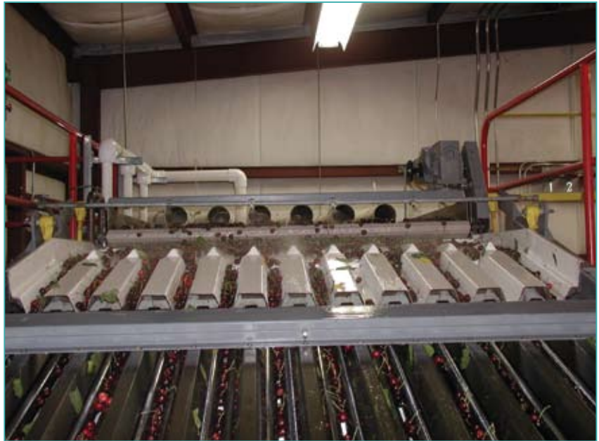
Cherries move through a bath of ozonated water at Orchard View Farms in The Dalles, OR. Working with green grocers like Costco and Tesco motivated the company to switch to an ozone system. Source: Novazone Inc.
